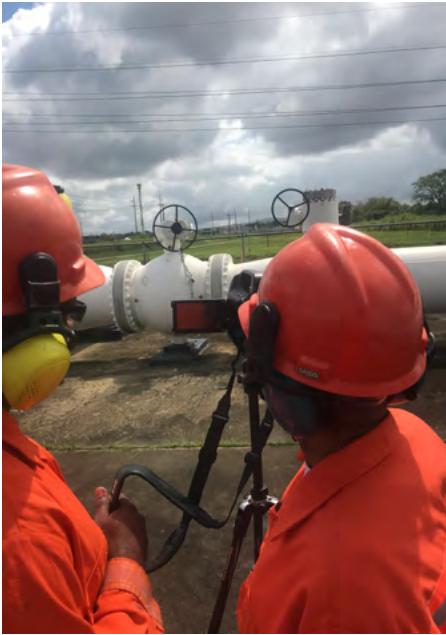
DRAFTED INTO USE IN FEBRUARY 2021, THIS CAMERA IS CURRENTLY BEING USED TO EXECUTE AN ANNUAL LEAK SURVEY ACROSS NGC'S ABOVE-GROUND INSTALLATIONS.
