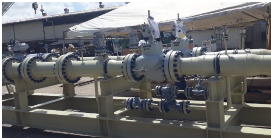
SECTION OF PRESSURE REGULATOR SKID PACKAGE AT FABRICATION YARD
