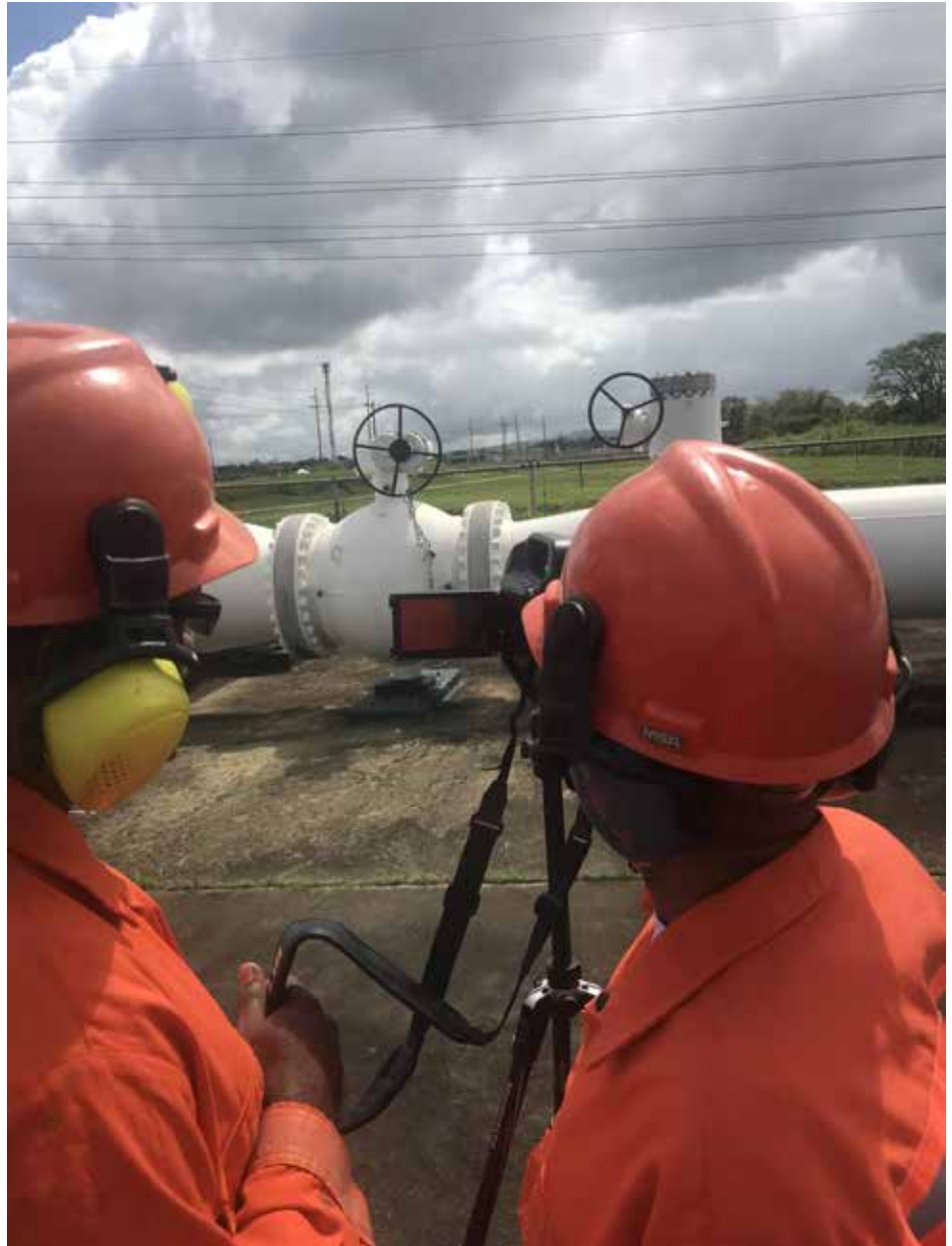
An infrared camera is helping NGC visualise leaks along its lines
