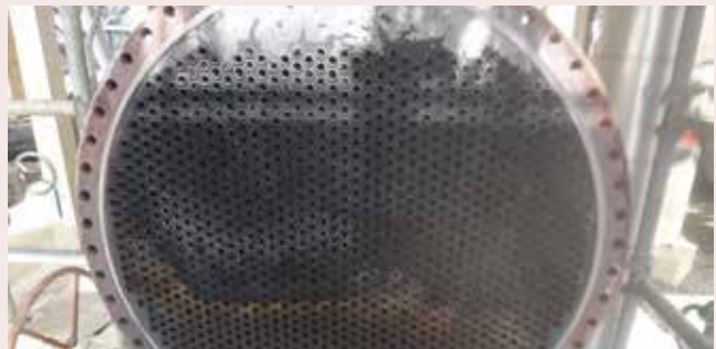
Fouled/plugged Exchanger tube bundle during cleaning process
